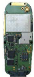
Radio Unit Application CPU Access CPU
